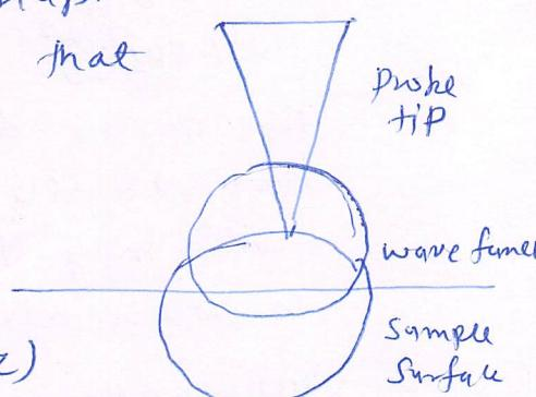
: Probe and Sample overlap wave function
